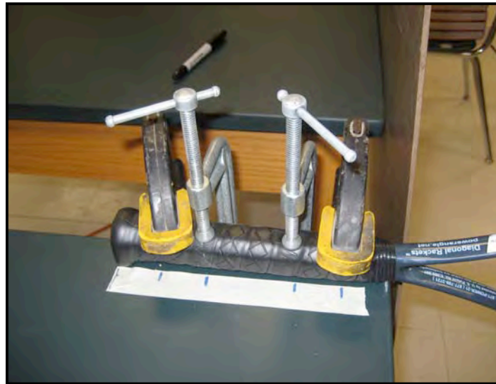
Figure 3.3 The method used for the clamping of tennis rackets during testing of both ball control and power. Four clamps were placed 1 cm and 4 cm away from both the top and bottom of the grip of each racket.
