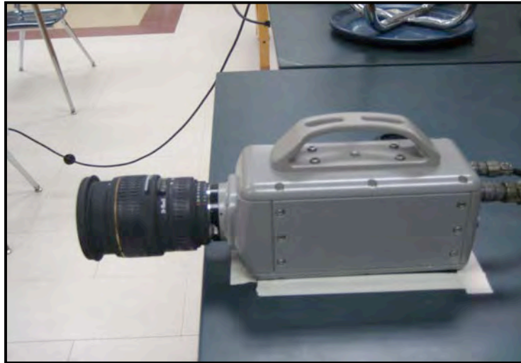
Figure 3.6 The Phantom 7.0 high-speed camera used during testing.
