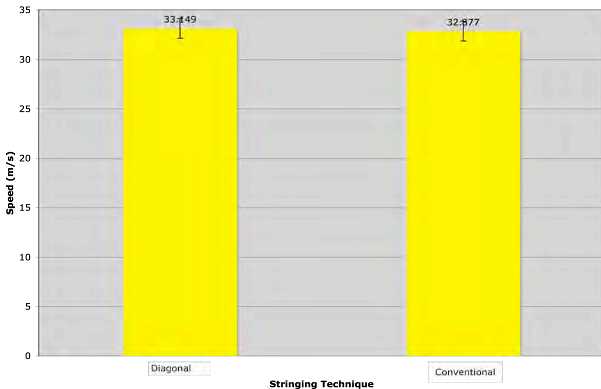
Figure 4.7 Comparison of power data for diagonally and conventionally strung tennis rackets. This variable was measured as the speed that the projected tennis ball left the face of the racket in each video. The number of frames necessary for the ball to travel 5 cm based upon the distance quantification grid in each high-speed video was used to determine this speed. Power Angle diagonal stringing was recorded as causing the tennis ball to need a mean of 10.86 frames (33.149 m/s), while conventional stringing caused a mean of 10.95 frames (32.877 m/s) ( p -value = 0.431). Error bars show the range of power findings.
